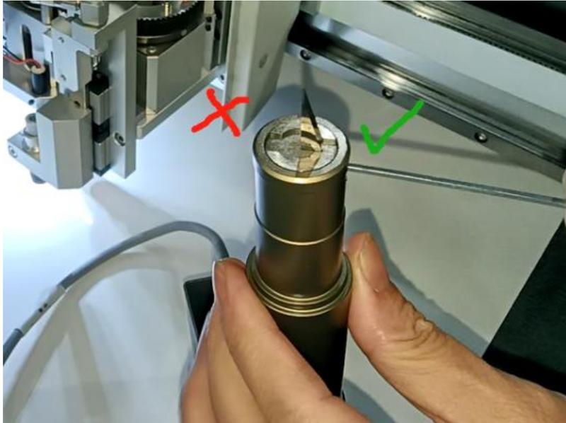
Remove the broken blade and insert the new one. Shake it with your hand to confirm it is inserted completely. Notice the direction of the blade.
