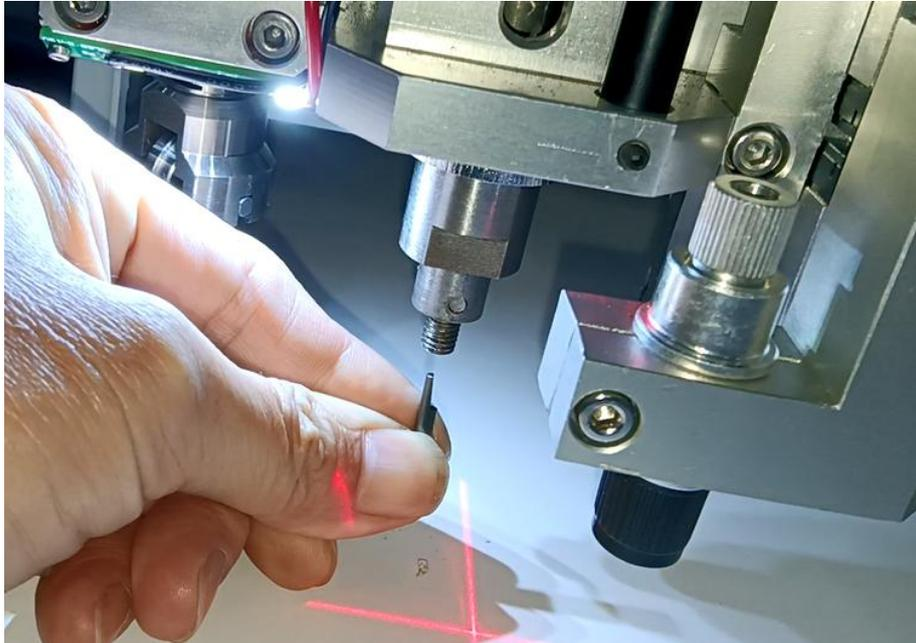
Put on the cap on the tool, turn it to adjust the length of the blade coming out to get half cut or full cut. When you adjust it, you can touch the blade with a finger.
