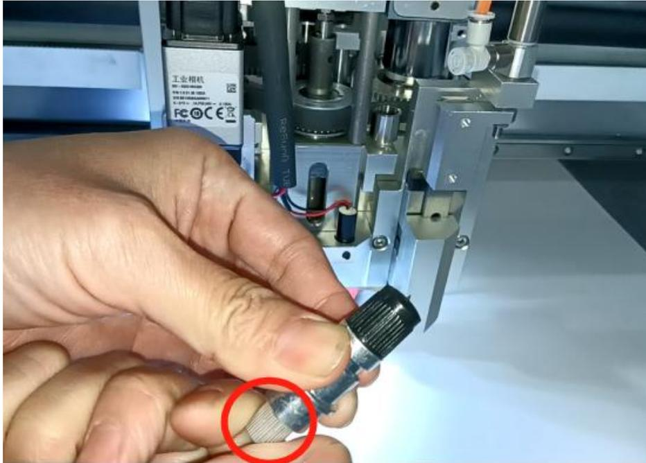
Put the tool on the holder and tighten the screw.
